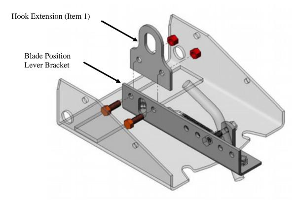
2. Attach the hook from the winch to the new mounting location on the Hook Extension..
