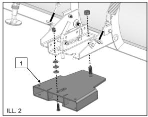
Torque rear bracket fastener to specification and adjust pivot nut to desired hinge plate freeplay.
