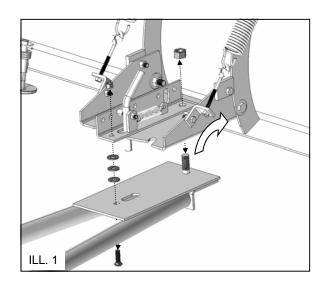
Place the QAB Weldment, Item #1, onto the hinge plate assembly. Insert spacers and fasten QAB with lock nut, carriage bolt, and pivot nut. See Illustration 2.
