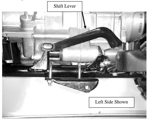
3. Place the attaching bracket onto the four u-bolts and secure with nylock nuts. The attaching bracket should be against the bottom of the ATV's mainframe tubes. Also be sure that the cutout hole in the attaching bracket is towards the back. See parts breakdown for proper orientation.
