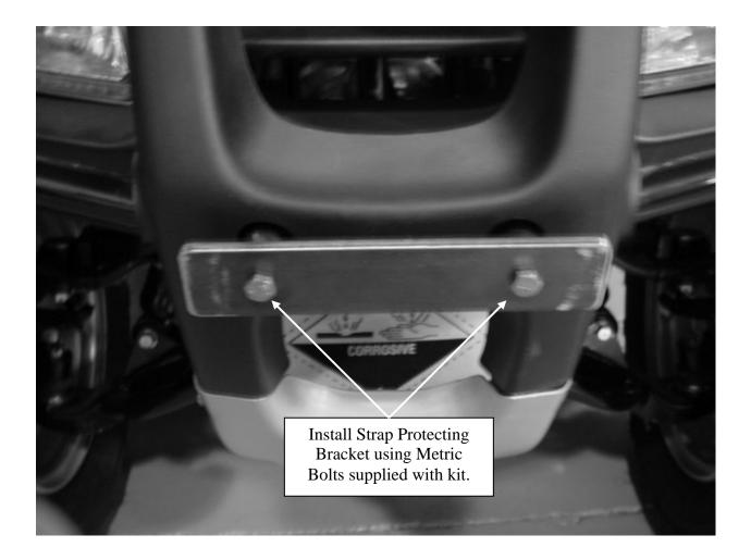
Included is a Strap Protecting Bracket pictured above. The bracket is designed to protect the front plastic grill from wear by the lift strap.
