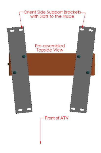
1. Pre-assemble attaching bracket (Item 1) and support brackets (Item 2) as shown in picture above using the four 5/16" x 3/4" carriage bolts and nylock nuts. **DO NOT FULLY TIGHTEN CARRIAGE BOLTS AT THIS TIME.**
