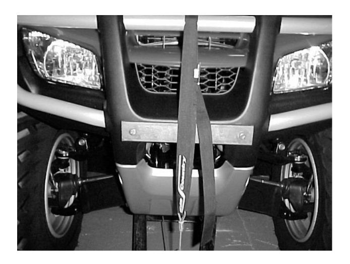
Included is a lift strap bracket pictured above. The bracket is designed to protect the front plastic grill from wear by the lift strap.
