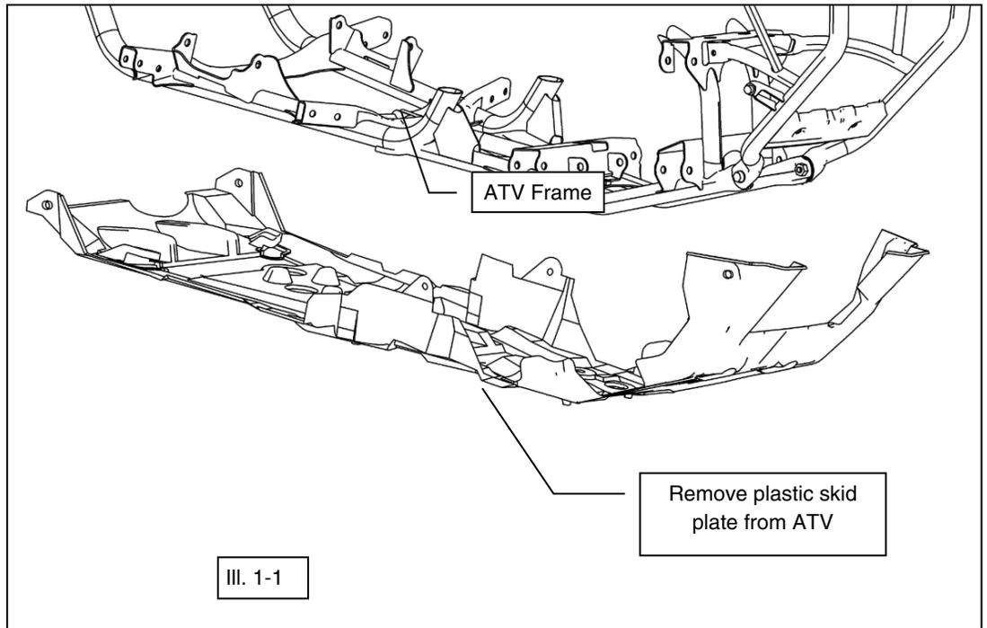
2. The plastic skid plate will need to be modified to be re-installed on the vehicle.
