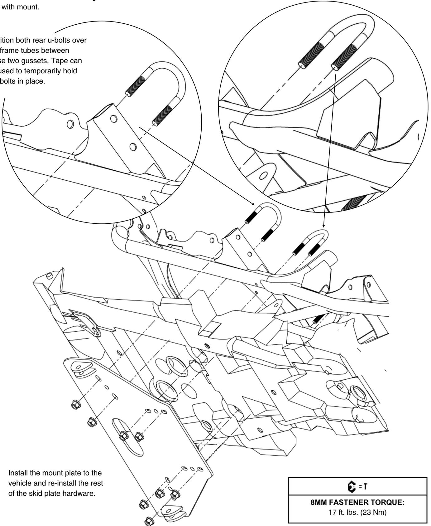
2. Install the mount plate to the vehicle and re-install the rest of the skid plate hardware.
