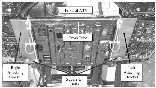
2. Center and attach the push tube to the attaching brackets. **Tighten lock nuts at this time.**
