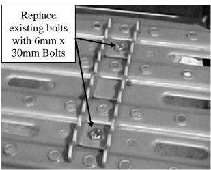
2. Hang the front of the attaching bracket onto the pan head bolts, loosely secure with the 1/4" nylock nuts. Swing the rear of the attaching bracket up to the metric bolts and loosely secure with the original nuts.
