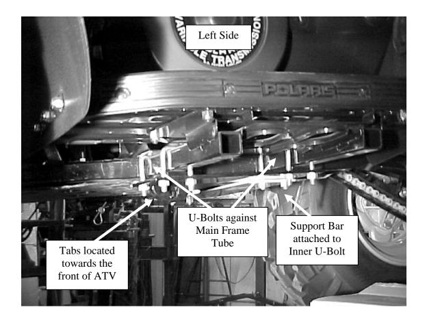
2. Place the other two U-bolts around the two, footrest support tubes and down through the two appropriate outside holes of the left push tube attaching bracket and loosely secure with the locknuts. **SEE PICTURE FOR CORRECT HOLES.**
