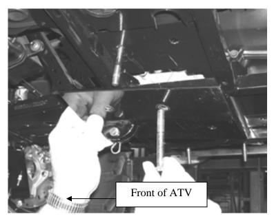
2. Install the two 3/8' x 3" bolts through the right backplate, open space opposite the left mounting bracket on ATV and through the right mounting bracket. Attach 3/8" nylock nuts. (*Do not fully tighten at this time*).
