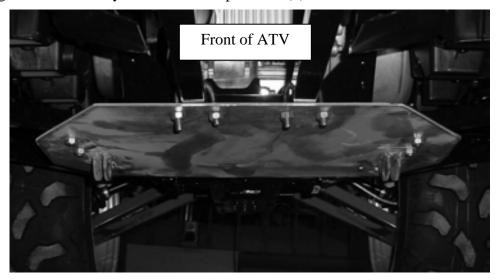
2. Tighten the rear two U-bolts first and then tighten the front two U-bolts. See Picture Below.
