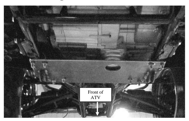
1. Place the four U-bolts provided over the frame and secure the blade mount weldment (Item 1) as shown in the picture above. Before tightening, be sure that the oil drain plug lines up with the cutout on the plate. If your ATV has a plastic skid plate, it may need to be trimmed.
