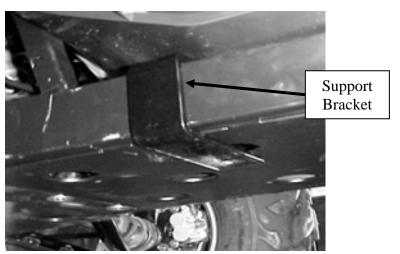
2. Place the main plate under the frame locating the U-bolt holes of the main plate on the square vertical tube as shown below. Start the two 3/8" x 1" bolts into the main plate and threaded support brackets. Do not fully tighten at this time.
