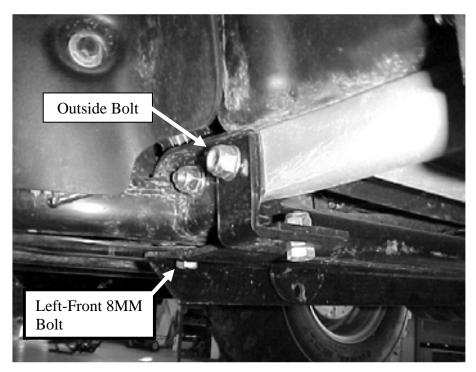
2. There are four (4) 8mm x 25mm bolts under the machine that hold the skidpan in place. Retain these for use when attaching brackets are removed. These will be replaced one at a time with 8mm x 30mm bolts
