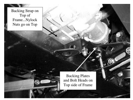
3. Lift the blade mount into position and attach to the backing strap and backing plates using the 5/16" x 2-1/2" bolts and nylock nuts provided.
