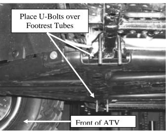
2. Align blade mount to U-bolts with the bent tab to the rear and down. Use flatwashers over slotted holes on plate. Mount so that the spacer blocks are positioned squarely over the foot rest brackets.
