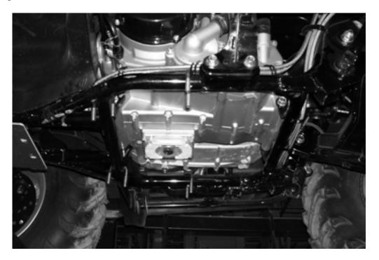
3. Align the hole on the blade mount weldment (Item 1) to the oil drain on the engine and install the blade mount weldment to the ATV frame using supplied hardware.
