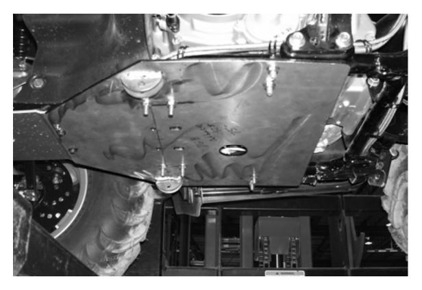
4. If the ATV has an aluminum skid plate, re-use the hardware to secure the front skid plate to the ATV using the slots provided in the blade mount weldment.
