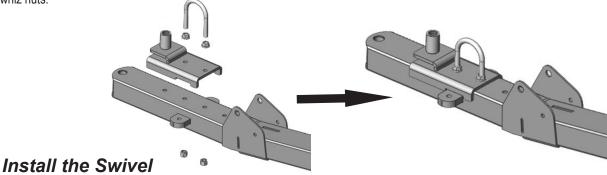
Slide the pivot tube spacer (W) into the hole in the front of the push tube and place the swivel (C) into position on the front of the push tube. The rear of the swivel will fit into the open groove of the swivel pin bracket. Align the front hole with the push tube hole and bolt in place through the pivot tube spacer using the 1/2" x 3-3/4" hex bolt (M), two 1/2" flat washers (N), and a 1/2" nylock nut (O). Swing the swivel back and forth all the way to ensure it rotates freely.
