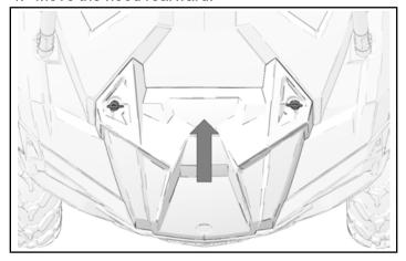
5. Turn the quarter-turn fasteners to lock the hood to the vehicle.
