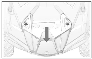
3. Remove and keep the two screws (a). Remove the winch cover.
