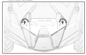
2. Move the hood forward to remove from the vehicle.
